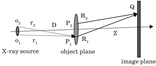
**Fig. 1.** Micro focus X-ray phase contrast imaging system diagram.
