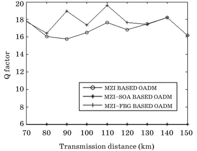
Fig. 7. Q-factor v/s Transmission distance plot of add channel at frequency 193.15 THz (ch-1) at -20 dB crosstalk.
