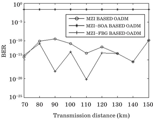
Fig. 8. BER v/s Transmission distance plot of add channel at frequency 193.15 THz (ch-1) at -20 dB crosstalk.
