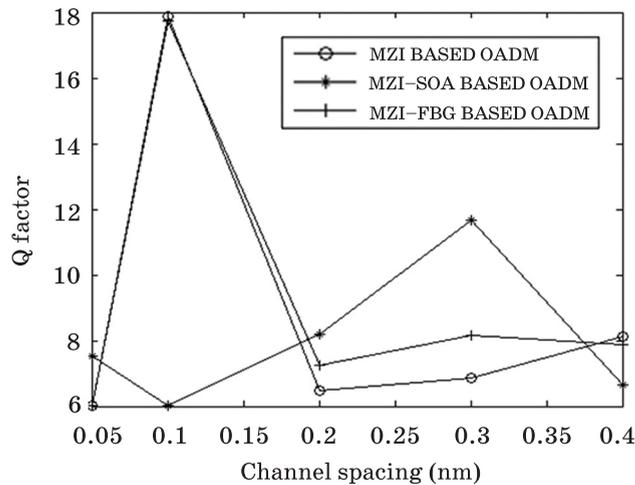
**Fig. 11.** Q-factor v/s Channel spacing plot of add channel (ch-1) at -20 dB crosstalk & 10 Gbps bit rate for 70 km.
