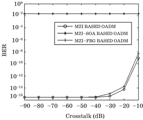
Fig. 6. BER v/s Crosstalk plot of add channel at frequency 193.15 THz (ch-1) for 70 km.
