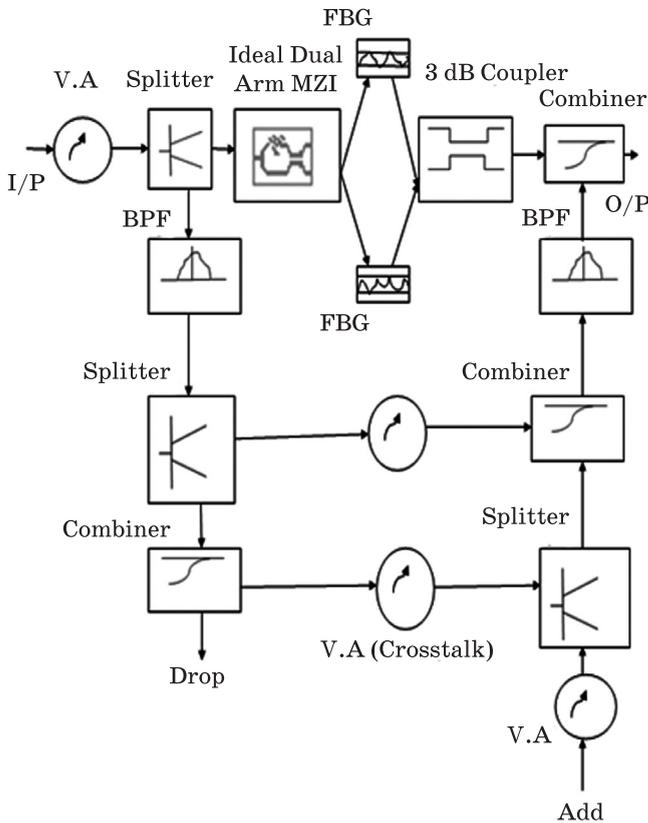
Fig. 4. Structure of OADM based on MZI-FBG.
