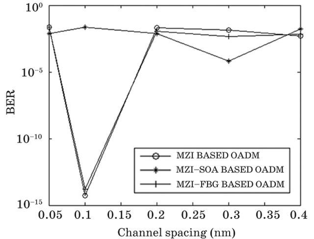
**Fig. 12.** BER v/s Channel spacing plot of add channel (ch-1) at -20 dB crosstalk & 10 Gbps bit rate for 70 km.
