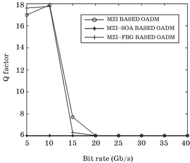
**Fig. 9.** Q-factor v/s Bit rate plot of add channel at frequency 193.15 THz (ch-1) & -20 dB crosstalk for 70 km.
