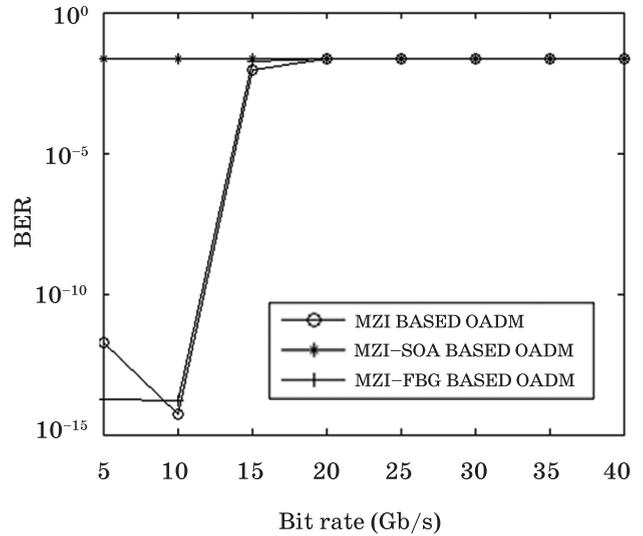
**Fig. 10.** BER v/s Bit rate plot of add channel at frequency 193.15 THz (ch-1) & -20 dB crosstalk for 70 km.
