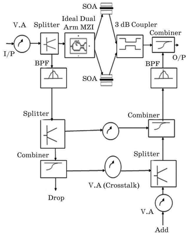
Fig. 3. Structure of OADM based on MZI-SOA.
