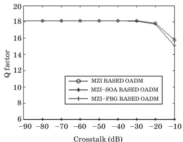
Fig. 5. Q-factor v/s Crosstalk plot of add channel at frequency 193.15 THz (ch-1) for 70 km.
