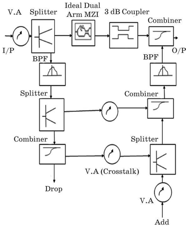
Fig. 2. Structure of OADM based on MZI.
