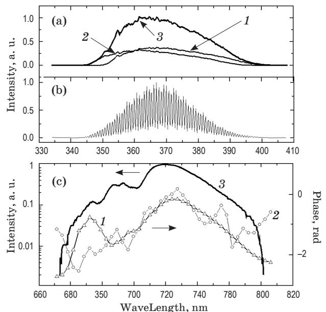
**Fig. 3.** Experimental interferogram (curve 3 –  $|\tilde{E}(\omega_1) + \tilde{E}(\omega_2)|^2$ ) and individual spectrums of up-converted replica in FISH (curve 1 –  $|\tilde{E}(\omega_1)|^2$ , curve 2 –  $|\tilde{E}(\omega_2)|^2$ )(a). Experimental interferogram in SPIDER (b). Experimental spectrum of the test pulse (curve 3), retrieved phases in FISH (curve 1) and SPIDER (curve 2) (c).
