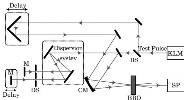
**Fig. 2.** FISH experimental setup: KLM – Kerr Locked Mode Ti: sapphire oscillator, BS – beam splitter, dispersion system – grating pair (1200 grooves/mm), M – mirror, CM – concave mirror ( $f = 100$  mm), DS – double slit aperture, BBO – up-converting Barium Boron Oxide crystal ( $30 \mu\text{m}$ , type II), SP – spectrometer.
