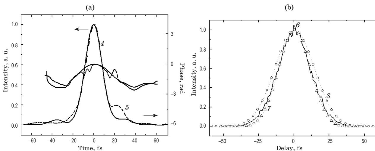
Fig. 4. Temporal intensity and phase in FISH (curve 4) and SPIDER (curve 5) (a). Experimental autocorrelation curve (curve 6), theoretical autocorrelation curves calculated from FISH's (curve 7) and SPIDER's (curve 8) experiment (b).
