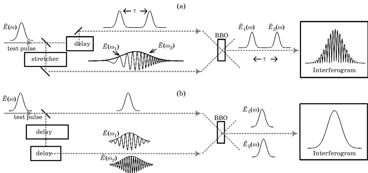
Fig. 1. Schematic of SPIDER (a) and FISH (b).
